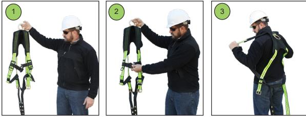
1 Hold harness by back D-ring. Shake harness so that straps fall into place.
